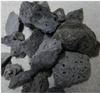
Fig. 1 Appearance of CA aggregate
