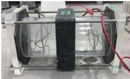
Fig. 1 Test equipment for unsteady-state electrophoresis test
