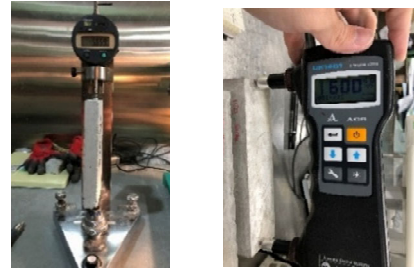
Fig.2 Equipment for dimensional change measurement (left) and UPV test (right).
