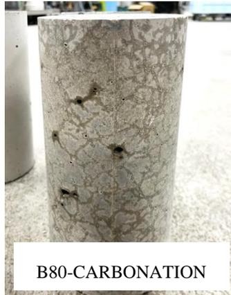
**Figure-4.** Microcracks of concrete
