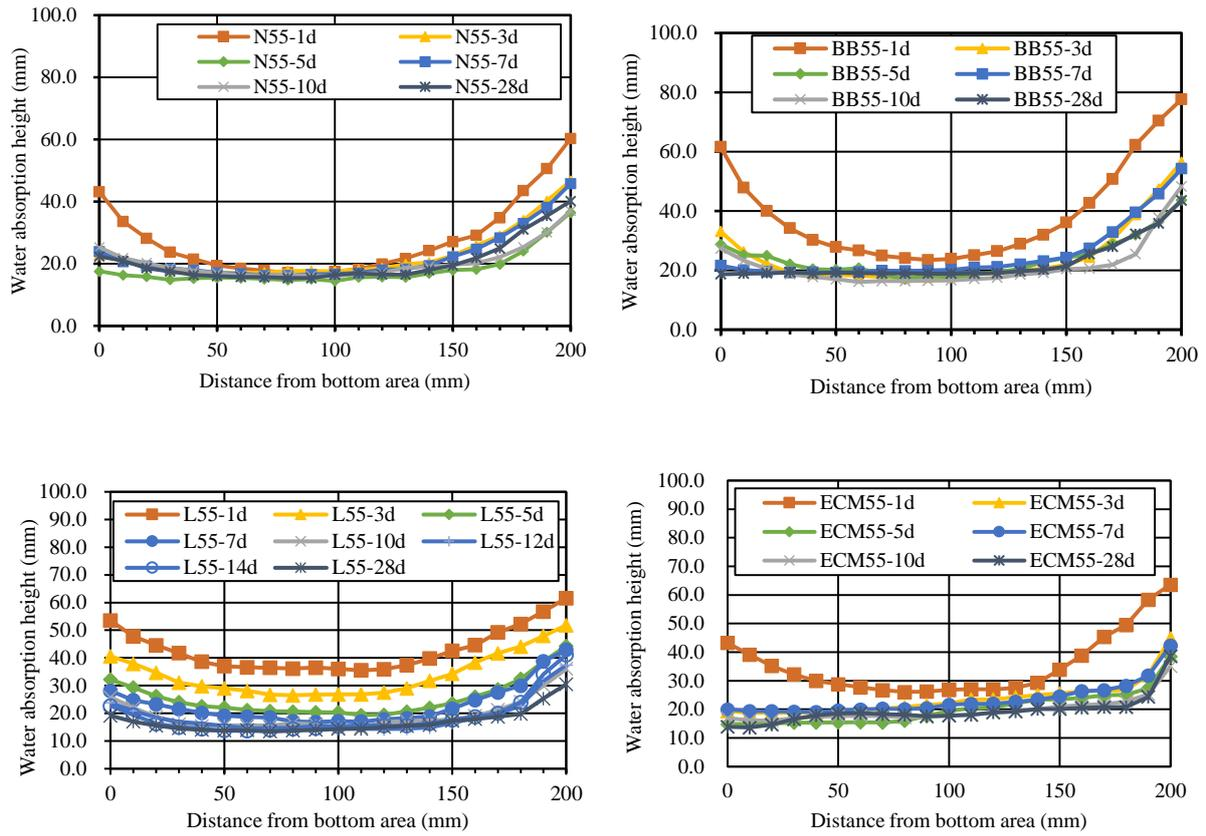
Figure 5 The results for water absorption test in vacuum conditions
