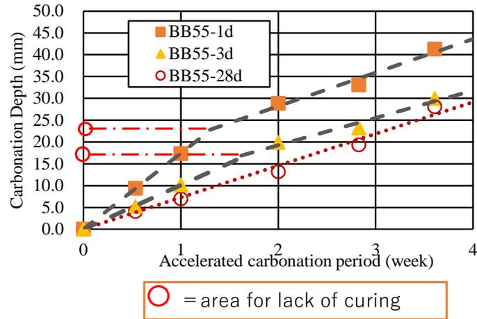
Figure 4 Carbonation Depth on accelerated carbonation periods on different curing period
