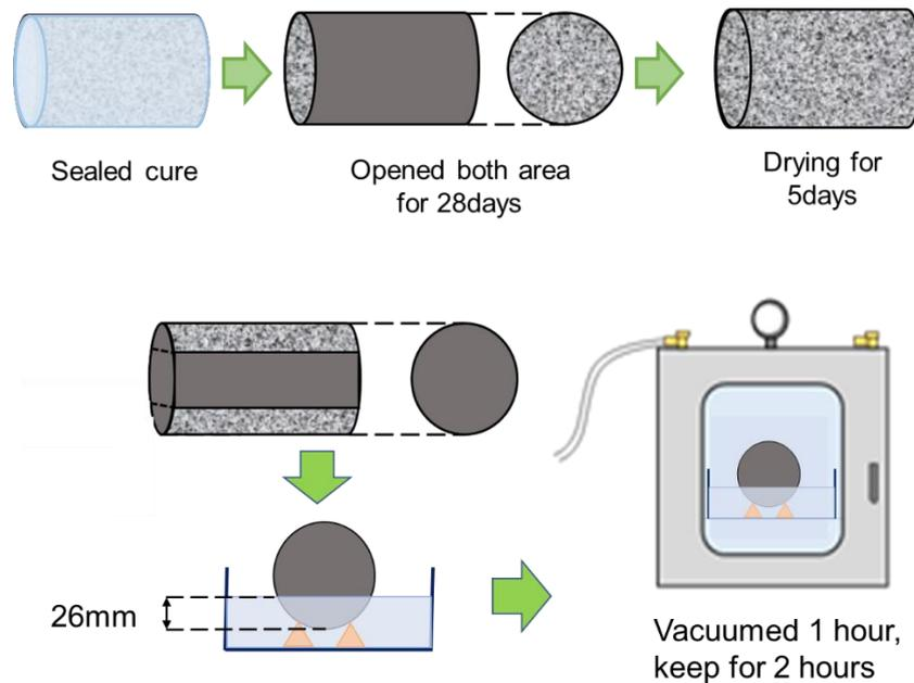
Figure 1 Testing methodology for vacuum absorption test
