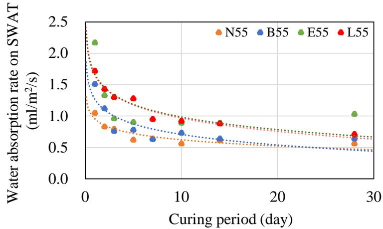
Figure 6 The results of water absorption rate in SWAT on different cement
