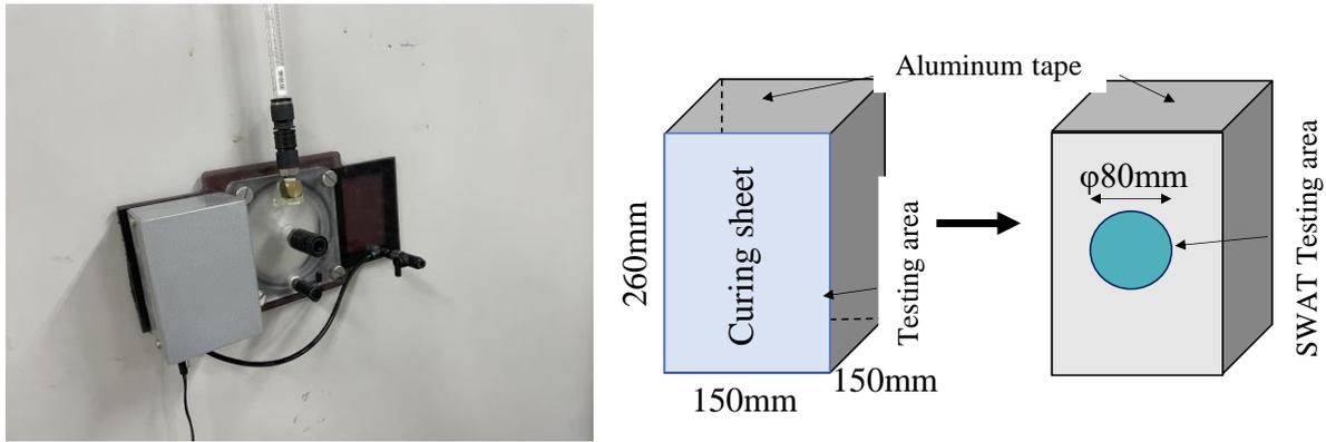
Figure 2 system for SWAT and outline of specimen
