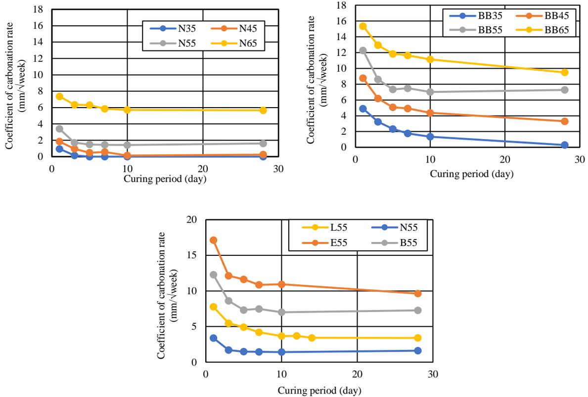
Figure 3 The results for coefficient of carbonation rate on different cements and W/C
