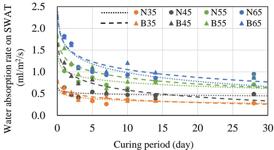
Figure 7 The results of water absorption rate in SWAT on different W/C
