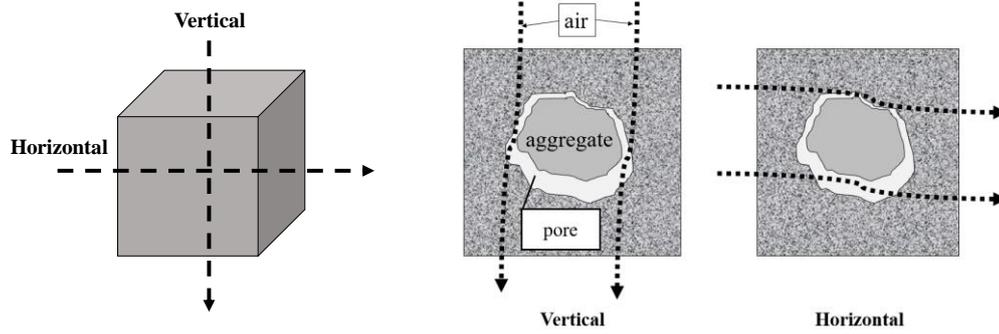
Figure 1 Core removal from different directions
