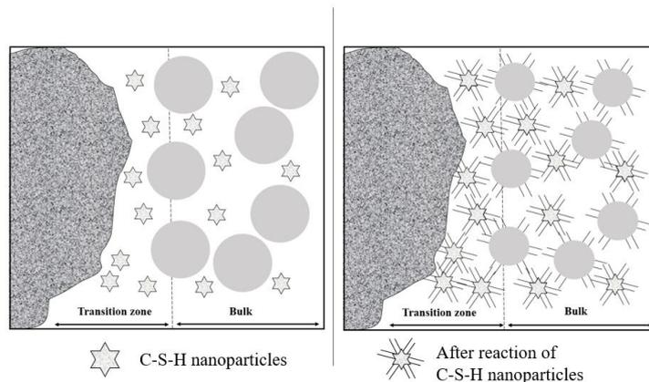
Figure 10 The function of C-S-H type accelerator
