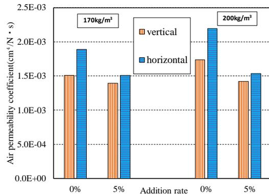
Figure 8 Air permeability test from different directions
