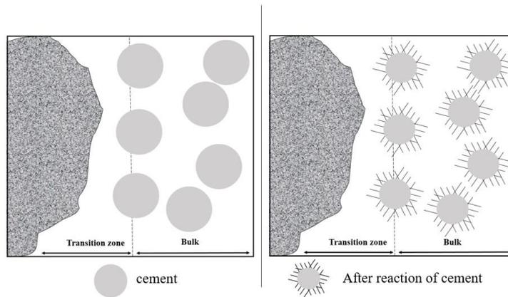
Figure 9 The hydration reaction of cement
