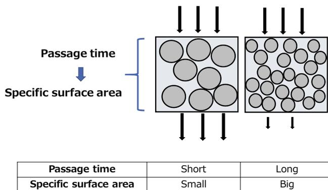
Figure 2. Measurement Principle of the Brane Penetration Device
