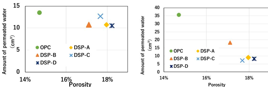
Figure 15 Relationship Between Amount of Permeated Water
