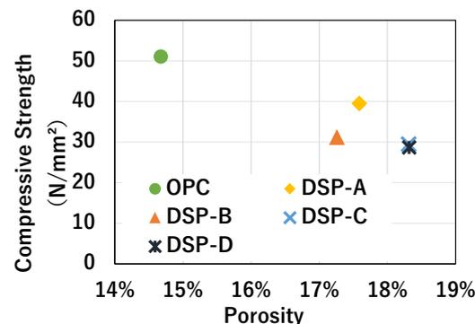
Figure 9. Relationship between compressive strength and porosity
