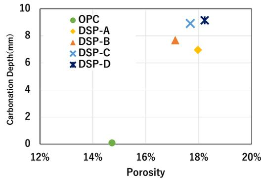
Figure 11. Relationship between Carbonation depth and porosity
