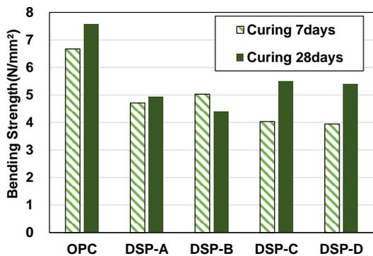
Figure 6. Result of Bending Strength
