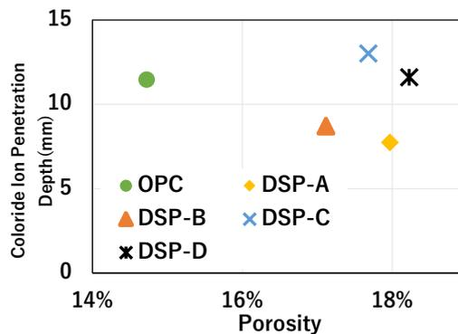
Figure 13. Relationship between Chloride Ion Penetration and porosity
