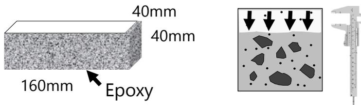
**Figure 5. Salt Water Immersion Test Method**
