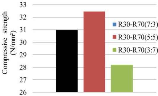
Figure 3. The compressive strength of the partial replacement of RCA (R30 & R70).
