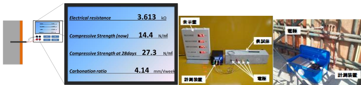
Figure.16 System for prediction of concrete properties in formwork using electrical resistance
