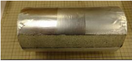
Figure 6. Sample of water absorption test in vacuum
