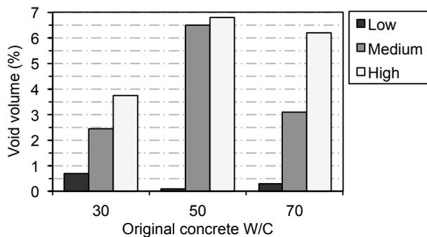
**Figure 7: Calculated void volume by W/C and mortar volume**
