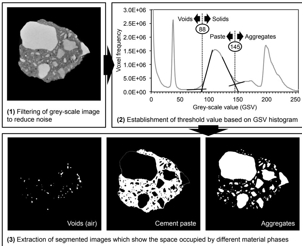
**Figure 5: Segmentation method for identifying different material phases**
