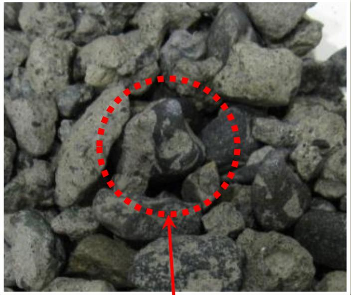
Residual mortar attached to aggregate
