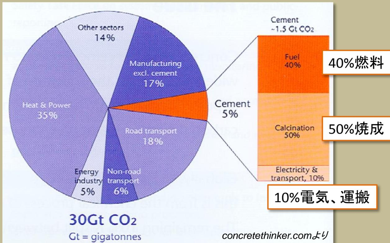
Cement used in concrete is responsible for roughly 5% of global CO<sub>2</sub> emissions
